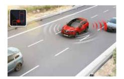
Blind spot warning This system detects the presence of vehicles in your blind spot. It automatically alerts the driver using a light signal located on the front left or right door mirror.
