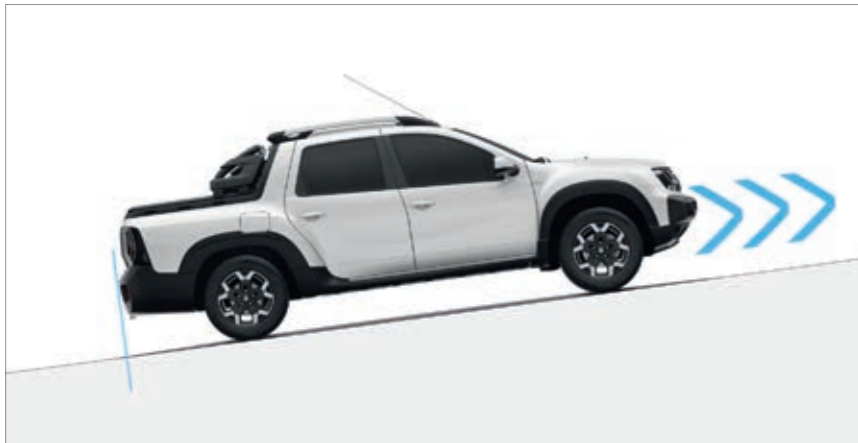
hill start assist Maintains brake pressure for two seconds, preventing roll-back when you move away on a steep slope.
